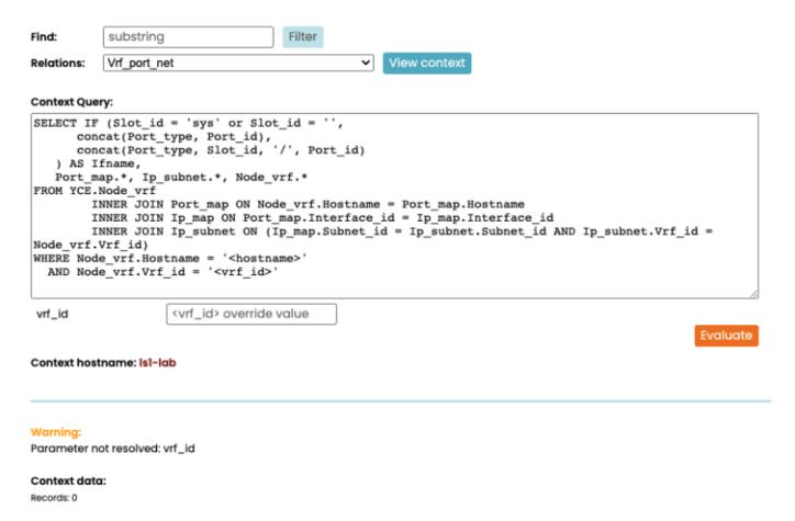
In the example above, the Relation uses a variable in its query that cannot be substituted directly from the nodes context and therefore prevents the query to retrieve data. The orange "Warning" informs that the Parameter <vlan> could not be resolved.
